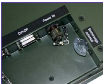
RD24 circuit breaker switch
